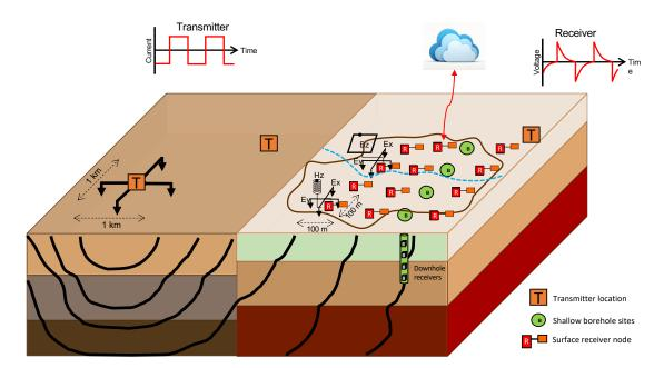
Figure 1: Controlled Source EM survey layout showing transmitter, receivers, and shallow borehole sensors. Each sensor can have muli-components in electric and magnetic fields as well as 3-component seismic sensors. The contour lines represent lines of equal current densities for progressing time.
